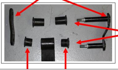
A center sleeve may or may not be required at this point in the bushing kit as some bushings may run directly on the shackle pin or spring eye pin.
