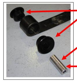
Install the supplied bushings into the spring eye or chassis eye.
