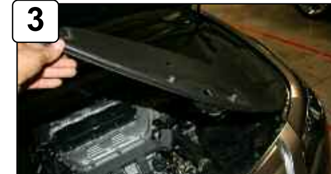
Remove all driver side plastic engine covers.
