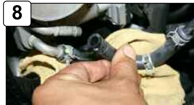
Remove crank case line attached with throttle body coolant line. Have a towel or rag handy to catch any leaking coolant. Use pliers to remove both lines. Save small clamps for later install. Caution: Coolant will leak from line when removing!
