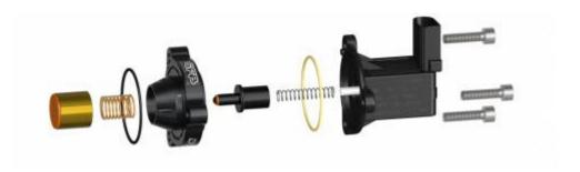
For the earlier DV+ T9351 models, all that is required is to replace the existing plunger and OE plunger spring with the parts supplied in the GFB upgrade kit.
