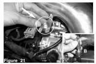
A)Install the primary intake tube and secure to the turbo nut and fender washer B)Re-install the fitting from step10, this will allow for the engine cover install.
