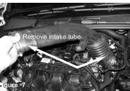
Carefully lift up and remove the stock intake tube from the vehicle.
