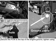
original 10mm screw. B)Locate the 1/4" hole on corner of heat shield. This will be used on 2015-16 model ST. C)With provided M6 screw and fender washer, install heatshield and secure to thredded insert from previous step. Use nylon spacer between heatshield and frame. Secure and tighten
