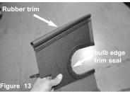
Install the bulb edge trim to the cut out on heat shield. Install the rubber trim to the top of the heat shield.
