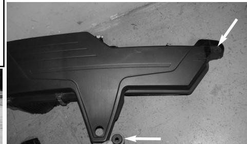
Remove the two factory mounting grommets from the OE air box assembly. These two grommets will be re-used later in the Injen intake kit.
