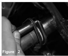
Remove the entire stock exhaust from the axle back. remove the 2 bolts and springs and save for install.
