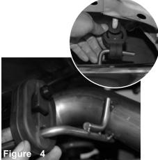
Install and secure the hangars. Secure and tighten using factory springs/bolts. Secure using provided M8 nuts. Tighten and secure the exhaust. Your installtion is now complete. Check for clearance and positon for best possible fit. Thank you for choosing Injen Technology!
