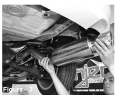
Install the Injen axle back exhaust, and position to the factory flange.
