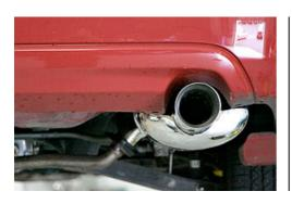
Get the two mufflers aligned up on the hangers so that the tips are in the middle of the exhaust cut-out area. Tighten the nuts and bolts up firmly at this time, and then adjust the mufflers again for a perfect fit.
