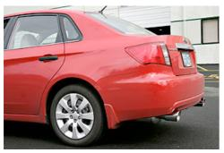
Make sure the vehicle is out of gear. Start it up, and then check the rear exhaust for any leaks while it is still up on the stands. If there is any leaks, turn the car off. Loosen the 14mm nuts on the flange, adjust the gasket, and re-tighten the nuts. Repeat the test.
