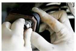
Insert the new AVO-supplied gaskets and bolts at the flange point. Then loosely hand tighten the bolts up at this time.
