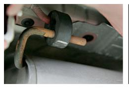
The stock mufflers will only be resting on the rubber hangers at this time. Spray some WD-40 or similar lubricant on the metal hangers where they meet with the rubber hangers. This will aid in removing them smoothly, especially if they are slightly rusty from age. Remove the two stock mufflers.
