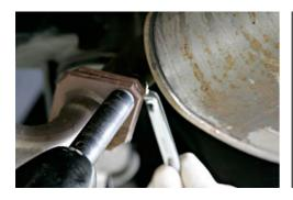
Using two 14 mm wrenches or sockets (or combination thereof), loosen the two bolts on the stock mufflers where they connect to the center y-pipe section. Remove the bolts and the factory gasket. Clean the surface of the two flanges on the center y-pipe to ensure a good fit.
