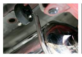
Spray some WD-40 onto the metal hangers of the AVO mufflers, and work them onto the rubber hangers.
