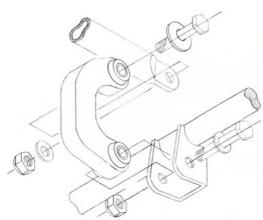
First remove the stock endlinks. This is done by removing the nut at the top where it connects to the stabilizer bar, and by unbolting the bolt at the bottom. Push the bolt out with a screwdriver.
