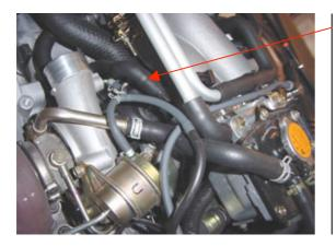
You will need to break the plastic fitting on the intake pipe, this will be enable you to remove the intake pipe under the inlet manifold. By pulling on the intake pipe towards the front of the car it can be removed this way
