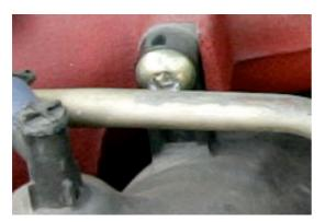
Remove the 12 mm bolt that mounts the intake pipe to the inlet manifold.
