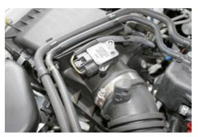
Lift the wiring loom up to allow easy removal of the intake pipe.
