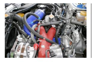
We have relocated the crank case breather hose from in front of the turbo to near the air box to allow easy fitting of the AVO pipe.
