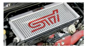
Remove the intercooler. Unbolt the two 12mm bolts on either side of the TMIC. Loosen the clamp on the throttle body/TMIC hose. Loosen the clamps on the TMIC hoses underneath the TMIC.
