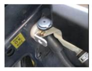
Once the stock airbox is removed, you will need to mount the bracket piece here. This is necessary for mounting Airbox Side A. From the front of the vehicle, it is to the left side, in front of the small engine cover piece on the left side of the engine bay. Mount Side A to the bracket.
