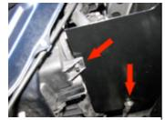
Airbox Side B is mounted to the body at the points indicated by the arrows, and should be connected to Side A by the supplied plastic Popits
