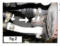
Unbolt the stabilizer bar end-link and the strut ball-joint at end of the control arm.
