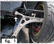
First you will need to remove the control arms from the vehicle. You will need to unbolt the front first. (Figure 1)
