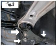
Unbolt the mounting brace from the vehicle first, and then unbolt the center nut from the Stud bolt.
