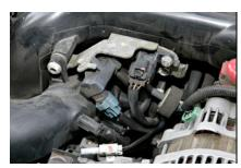
Remove this bracket and sensors. (take note of where the vacuum line goes)
