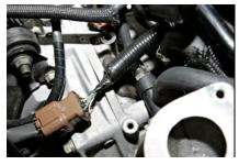
Remove the hose clamp off the intake pipe.
