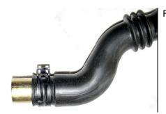
Fit the steel adapter pipe to the blow off valve return pipe
