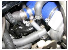
Fit the blow-off return hose to the blow-off valve intake pipe.
