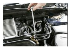
Remove the 12mm bolt from the intercooler mount.
