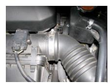
Remove the rubber intake pipe from the stock air box to the intake pipe
