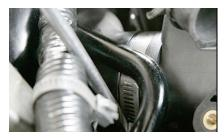
Remove the hose clamp on the intake manifold side of the intercooler
