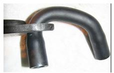
Trim the stock breather line at this point, and fit the supplied 13mm straight joiner.
