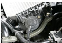
Remove the vacuum hose from factory Blow-Off-Valve (BOV)
