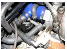
Fit the intake pipe to the turbo - tighten the hose clamp at the turbo end first.
