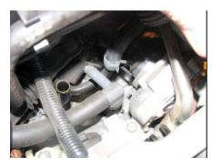
Fit the breather line from the front of the intake pipe to the crank case breather here:
