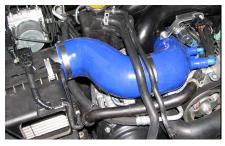
Fit the crank case breather line to the front off the intake pipe. If you are running a FMIC you can run it under the intake manifold. If you are running a TMIC you will need to go around the intake manifold.
