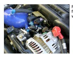
Fit the bracket and the sensors back to the intake manifold – it is a tight fit. Make sure the breather and vacuum lines are correctly fitted. You will need to add the t-joint as per the photo.
