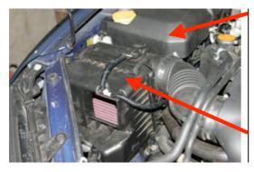
**Step 1** – Remove accessory cover behind air intake box.
