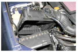
**Step 5** – Remove the stock air filter by pulling out towards the back of the car. Clean the bottom of the airbox.
