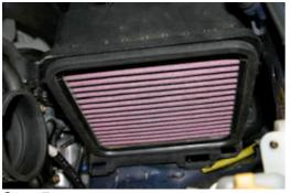
**Step 6** – Insert AVO air filter with the filter fins positioned horizontally – see photo.
