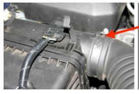
**Step 3 –** Loosen the clamp holding on the rubber air intake pipe.
