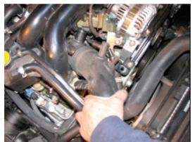
Remove the intake pipe by pulling it out the front.
