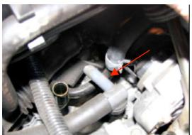
Fit the breather line from the front of the intake pipe to the crank case breather here:
