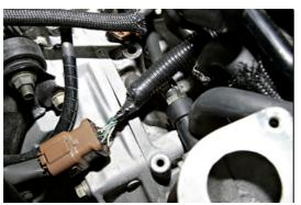
Loosen the hose clamp on the OEM inlet pipe.
