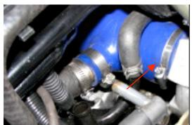
Fit the intake pipe to the turbo - tighten the hose clamp at the turbo end first.
