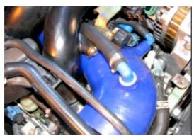
Fit the crank case breather line to the front off the intake pipe. If you are running a FMIC you can run it under the intake manifold. If you are running a TMIC you will need to go around the intake manifold.
