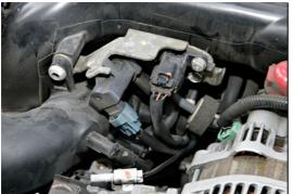
Unbolt this sensor bracket and keep it to the side during the install. Take note of where the vacuum line goes.
