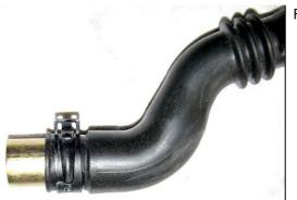
Fit the steel pipe to the blow off valve return pipe
