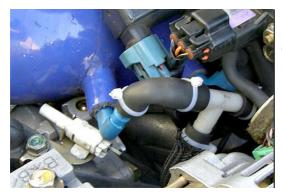
Fit the bracket and the sensors back to the intake manifold – it is a tight fit. Make sure the breather and vacuum lines are correctly fitted. You will need to add the t-joint as per the photo.
