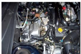
Remove the stock intercooler from the engine. You should cover the turbo compressor outlet with a clean rag to prevent any debris getting into the turbocharger while you are working.
