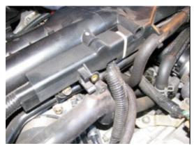
Remove the Blow off valve return hose from the intake pipe - you will need to remove this 6mm bolt
