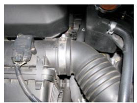
Remove the short rubber intake pipe that goes from the stock air box to the stock inlet pipe.
