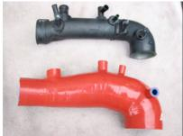
The AVO inlet pipe is quite a bit bigger and longer than the standard inlet pipe. It is designed this way for a variety of
