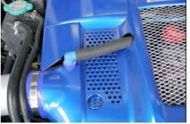
An alternative method for routing the crankcase breather hose is pictured here.
