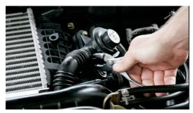
Remove **two** 10mm headed BOV retaining bolts that hold the BOV to the the factory intercooler.
