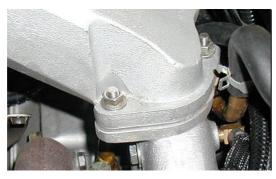
Remove the two 12mm nuts connecting the turbo to the intercooler (take care to not drop the nuts). On a stock intercooler this is a rubber o-ring used to seal the TMIC to the turbocharger, do not lose this.
