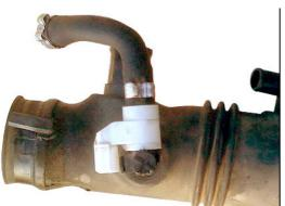
US Market Legacy models only: Remove this PCV sensor and hose from the inlet pipe. Unplug the wiring harness from it, and run a small wire across the two pins.
