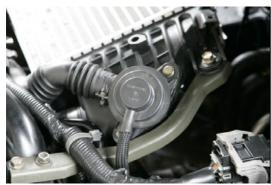
Remove the small vacuum hose from the top of the factory Blow-Off-Valve (BOV).
