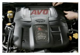
Remove 4 press-in retaining clips from the plastic upper engine cover. Removal of these clips requires a 1/2 turn counter-clockwise while applying very light pressure with a Phillips head screwdriver. Once the center pin pops up the clip can be removed. Remove Plastic engine cover.
