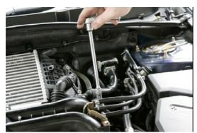
Remove the 12mm bolt from the intercooler mount bracket.
