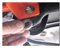
Take the washer from the bolt on the other side, and mount it between the bracket and the subframe, as the subframe has a slight inset. By using the washer in-between, it allows the brace to mount up flush against the subframe correctly.
