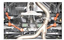
Make sure that you have left and right side underbody braces on the correct sides.
