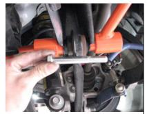
The rear underbraces will be connected here by the longer supplied bolts. The stock bolt is not long enough to fit them.
