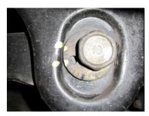
You will need to remove the nut on the other side of the rear undersuspension camber bolt to fit the rear braces. Make sure to mark the current position of the rear camber setting before you do so, as you will need to return it to this original position for correct rear alignment.
