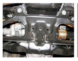
Remove all underbody guards and braces so that you can access the steering rack mounts.
