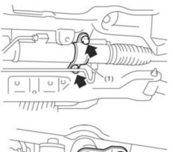
Undo and remove the steering shaft mount bracket bolts (top illustration), and the gearbox bracket bolts (bottom illustration).
