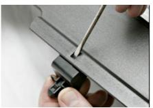
Finally, there are four clips at the top rear of the grill fastening it to the frame. These are easily removed with a small screwdriver. Simply insert the head of the screwdriver into the hole at the top of the grill.
