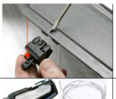
And press down on the tab inside the hole to slide the grill off. After the grill has been removed, remove these four mounts from the car, as they are no longer required. To remove them, push down on the small tab at the top near the body.
