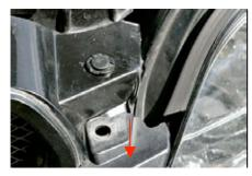
Remove the factory front grill from the car. There is two main pop-its holding the grill at the top, and small screws holding the grill from the back. The pop-it is easily removed with a small, flat-head screwdriver. The screws in the back need to be reached from behind. You may need to remove the two pop-its holding the bumper down (see arrow).
