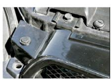
Once you have assembled the grill to your satisfaction, install it on the car. Insert the pop-its in the top opening on either side. You may need to place a bit of foam padding between the bumper skin and bumper beam to get the bumper to match up correctly at the bottom.
