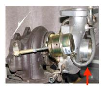
**Vacuum line** - Fit the black vacuum line that is hanging off the actuator to the turbocharger compressor cover directly - **DO NOT USE THE T JOINT** - make sure to clamp on firmly.
