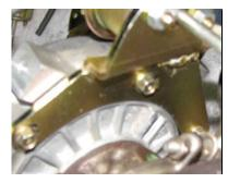
**Fitting the AVO actuator bracket-** with the actuator in place fit the three 5mm bolts tight, make sure the flapper valve is shut and the pin is over the actuator rod hole.
