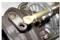
**Setting the rod length -** Fit the AVO Actuator to the recommended pre-load on the actuator spring. When it is in the correct position, it should look like this, slightly short of the hole. This ensures that the proper pre-load is on the wastegate.
