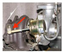
Use an air compressor gun to put air pressure into the actuator - until it reaches about 15 PSI. This will extend the rod and allow easy fitment to the turbo swing arm. Fit the original E-clip back in original spot and check the clip is secure.
