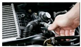
Remove **two** 10mm headed BOV retaining bolts from the factory intercooler.
