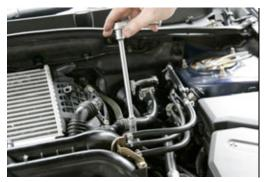
Remove the 12mm bolt from the intercooler mount.
