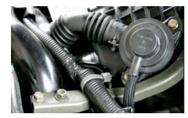
Remove the vacuum hose from factory Blow-Off-Valve (BOV)
