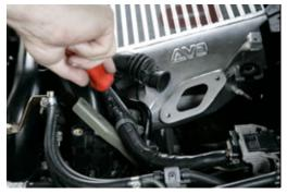
Tighten up the hose clamp on the intake manifold side.
