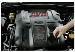
Fit the engine cover - use the 2 x BOLT-003 (6mm x 20mm) bolts with the washers at the **rear** of the engine cover and the **standard clips** at the front of the cover.
