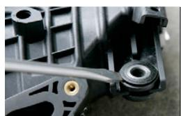
Remove the rubber grommet from the stock intercooler.
