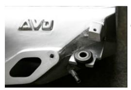
Fit the rubber grommet to the AVO intercooler.
