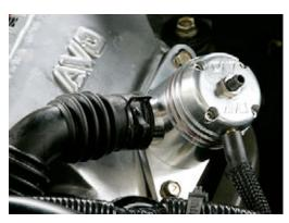
Fit the BOV tight – torque the two 6mm bolts to 8.8N.M.
