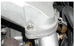
Start by tightening up the **turbo side bolts**, then the **mount bolt** near the BOV. Tighten to 21.6N.M with a torque wrench.
