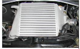
Fitting the intercooler: **Start** by pushing in the **intake manifold side onto the throttle body hose**, then line up the **turbo side**.
