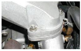
Remove the 2 12mm nuts connecting the turbo to the intercooler (take care to not drop the nuts)
