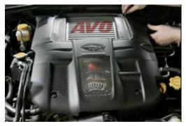
Remove 4 press-in retaining clips from the plastic upper engine cover. Removal of these clips requires a 1/2 turn counter-clockwise while applying very light pressure with a Phillips head screwdriver. Once the center pin pops up the clip can be removed.
