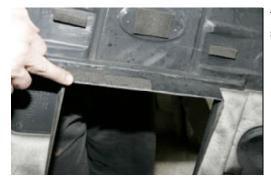
The engine cover will require some minor trimming at the front side off the cover. You can use a box knife to do this (test fit)
