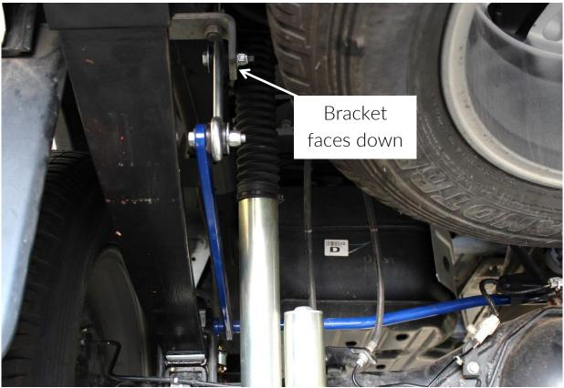
Figure 1 - Sway bar installation.
