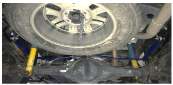
Figure 4 - Sway bar installation.
