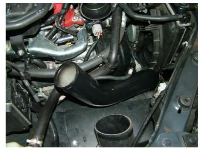
Next install this silicon hose from the intercooler to the above pipe.
