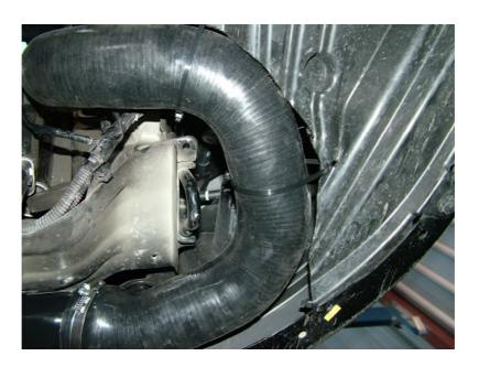
Re-install under tray. To install the under tray you will need to cut some plastic to give clearance for the new intercooler pipes.
