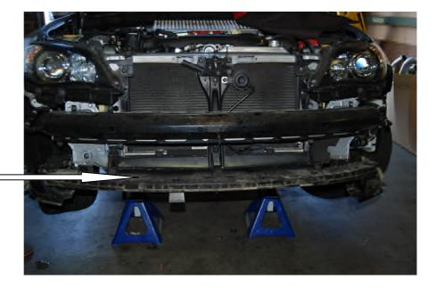
now remove this steel panel..to do this you will first need to unplug the headlight washer hose from each end
