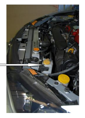
To give clearance for the intercooler piping you will need to bend this air conditioning line a little. This pic shows before..next pic after.
