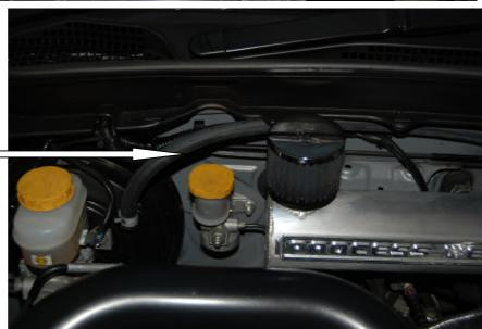
Connect the hose into this factory hose. Be sure to leave this hose in place as it has a one way valve inside it that is crucial for the brake to work correctly
