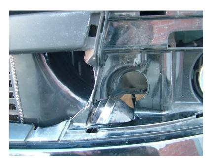
Once enough plastic has been removed the front bar will "click" back into place without any pressure on the bar itself.
