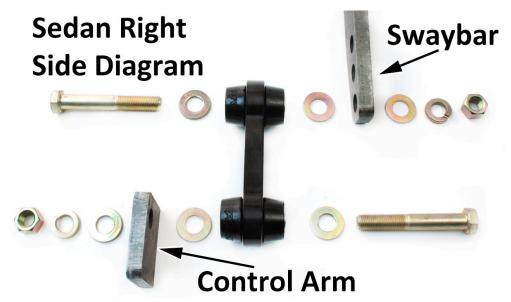
b. If you have a Wagon or 93-00 Impreza follow below picture. First you will need to drill out holes in control arm to 3/8" This is done to accecpt supplied 3/8" bolt. Place endlink between both tabs on control arm and install supplied bolt. **NOTE: Apply a small amount of grease to both sides of endlink bushing that touch each side of control arm.** Install supplied 3/8" flat washer, then 3/8" lock washer, then 3/8" nut to secure endlink to control arm. Leave loose at this time.
