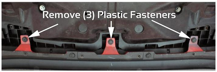
d. Under the bumper, on both the left and right sides, locate and remove (3) additional plastic fasteners.
