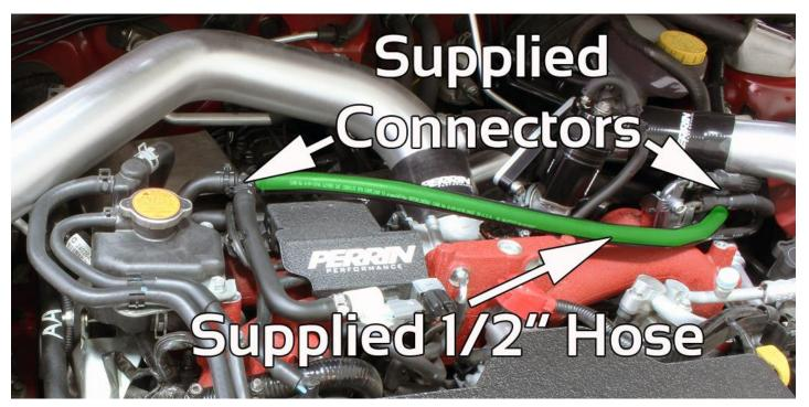
31) Install coolant reservoir. See instructions included with ASM-ENG-500 for installation of coolant overflow tank. Follow the directions for the vehicle you have. You can use the instructions for other years if you choose to do a custom install or have other parts installed that may affect the installation of the PERRIN Coolant Overflow.
