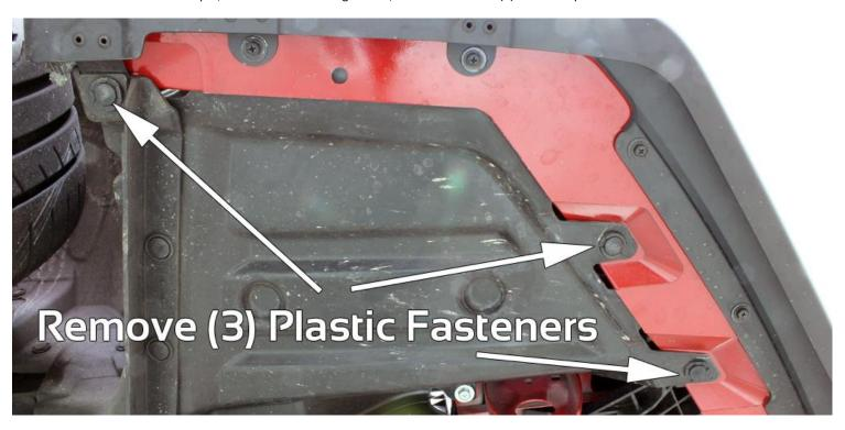
e. Grab right side bumper where plastic push connector was, and pull straight away from car. Do this until most of the right side has come off, then do this to the other side. There should be enough length of wire (from the fog/blinker lights) to set bumper on the ground. Unplug each connector as shown below.
