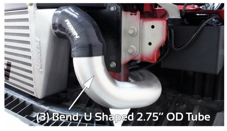
15) Install (3) Bend U Shaped 2.75" tube on left side of intercooler as shown. Use supplied 48 size clamp to secure to 90 degree coupler. **NOTE:** Adjustments to boost tubes will be made in later steps.
