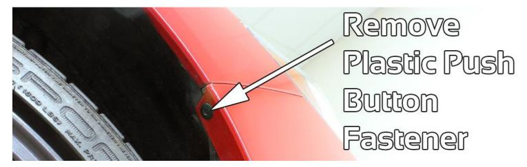
c. Under the bumper locate and remove (3) plastic fasteners in center of bumper.
