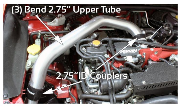
26) Adjust the rotation and length that tubes are pushed into the couplers. Adjust tubes so they do not hit on the engine, and/or other parts of the car that will cause damage to the tubes. Tighten all T-bolt clamps. **NOTE: These may need to be adjusted one more time before the install is complete.**
