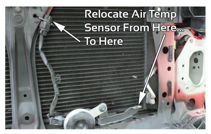
10) Locate horn on right side of car, loosen bolt and rotate out of the way as shown below. This is done to make room for boost tube to pass through.
