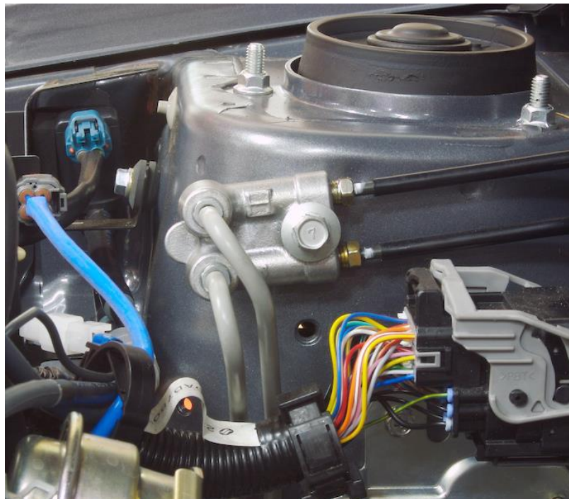
Shows Brake Line Junction Relocated, a very important step!
