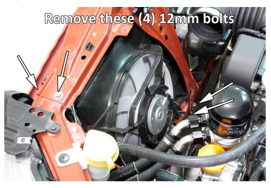
8. Lift up on left side of radiator support (leaving intake air diverter in place) and place PERRIN intake tube under support as shown below. Make sure that tab on PERRIN intake is in front of radiator support and closely lines up to threaded M6 hole shown below. Carefully set radiator support back down and reinstall (4) 12mm bolts removed earlier.
