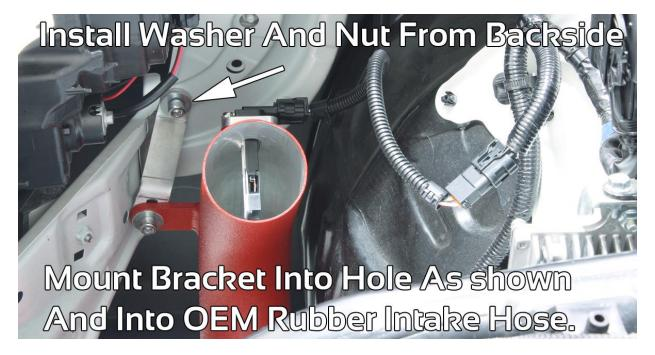
13. Mount lower portion of intake to chassis using M6x40 bolt, M6 fender washers, M6 nut and a single spacer (as shown below) into upper hole in bracket on PERRIN intake (making intake sit lower in chassis). Leave slightly loose for now.
