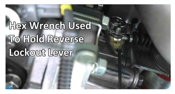
4. Inside of vehicle, 1/8" punch, carefully drive pin from OEM reverse lock out lever. With pin removed, slide reverse lock out lever off shifter. **NOTE: When** hammering pin out, push forward on the shifter in 1st, 3rd, or 5th gear and hold some tension on the shifter.
