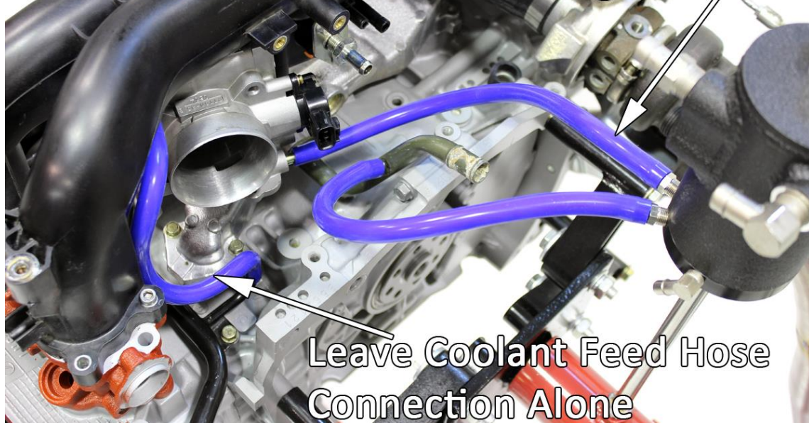
2008+ WRX coolant hose routing shown above. Diagram shows simplified path to help visualize routing.
