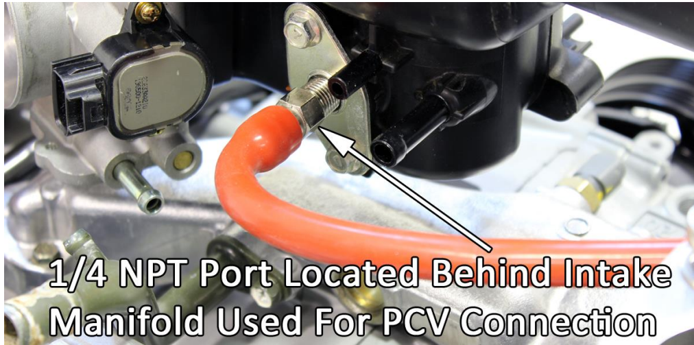
Above picture shows PCV port on 2008-14 WRX manifold.
