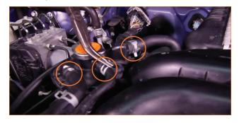
06. Remove the bolt that holds the expansion tank in place.
