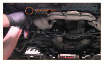
**04.** Tighten the petcock on the radiator once the coolant has drained below the expansion tank.
