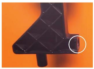
23. Install the Mishimoto mounting posts onto the Mishimoto radiator using the supplied hardware. Snug these bolts, but do not fully tighten them. (4x 10mm bolts)
