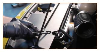
**05.** Compress the spring clamp that secures the overflow hose to the driver-side corner of the radiator and slide the clamp up the hose. Then pull the hose off the radiator.
