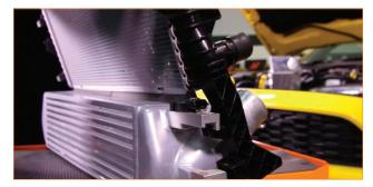
21. Remove four clip-nuts from the stock radiator and transfer them to the Mishimoto radiator. (4x clip-nuts)
