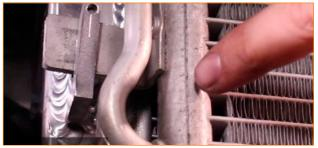
43. Align the upper mounting pegs with the isolators and slide them in. Then secure the radiator cradle with the four original bolts. (4x 10mm bolts)
