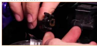
28. Release the quick-disconnect clip that secures the upper radiator hose to the radiator. Then work the radiator hose off the radiator. This connection can be very tight, so take your time to avoid damaging the hose connection.
