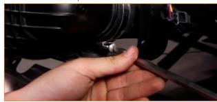
**19.** Loosen the clamp on the cold-side intercooler coupler, and disconnect the coupler from the intercooler.
