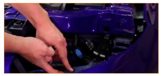
14. Remove the upper air shroud by releasing the two clips.
