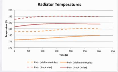
**Figure 7**: Overall coolant temperatures are lower with the Mishimoto unit. Pure distilled water was used for all tests. If a 50/50 mixture is used you can expect to add around 10°F to all plots.
