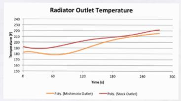
Figure 11: Mishimoto radiator revealed overall lower outlet temperatures when compared to the stock
