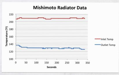
Figure 8: Highway test of stock radiator
