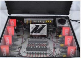
**Figure 2**: PLX devices in portable case used for testing Mishimoto products
