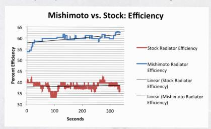
Figure 10:Comparison of efficiency between the stock and Mishimoto radiators. Notice that the Mishimoto radiator on average is approximately 20% more efficient than the stock radiator. This proves that the Mishimoto radiator has a higher capacity to keep the M3 running cooler.
