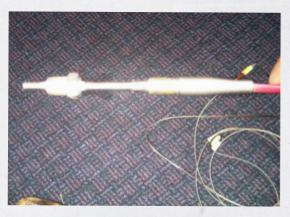
Figure 4: A thermocouple was mounted in the grille of the M3 to measure the temperature of the air as it entered the system. (Above image is of the K-type thermocouple used for measuring air temperatures.)
