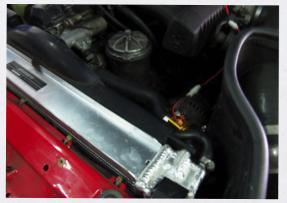
Figure 1: Fluid temperatures were taken from the inlet and outlet of both radiators using Mishimoto inline water temperature sensor adapters and PLX fluid temperature sensors. (Inlet sensor location is shown above.)
