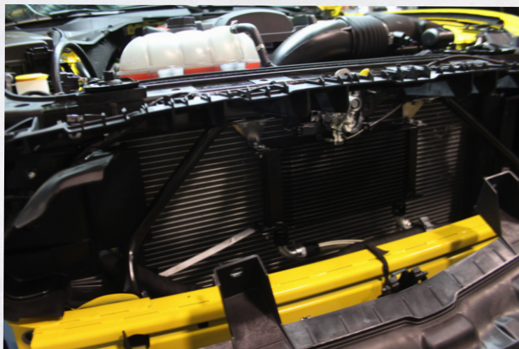
Figure 4: The upper-central location of the oil cooler allows a sufficient amount of ram air to enter the cooler without blocking airflow to the charge air cooler.
