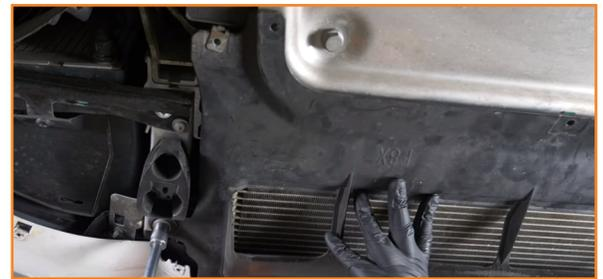
3. Loosen the bolts that secure the oil cooler brackets. (3x 13mm bolts)
