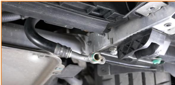
12. Install the Mishimoto oil cooler using the original hardware. (3x 13mm bolts)
