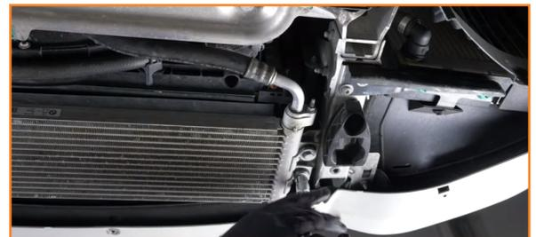
4. Remove the nuts that secure the lines to the oil cooler. (2x 10mm nuts)
