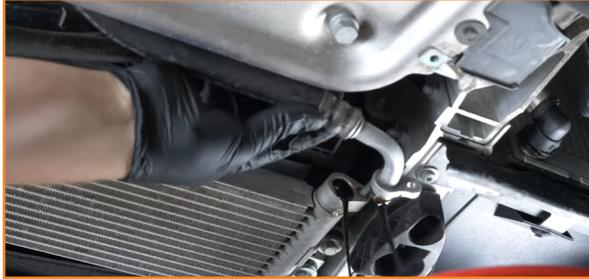
7. Release the loose bolts on the passenger side to let the cooler drain. Lean the cooler over the bucket so the remaining oil drains out.
