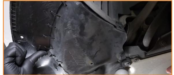
2. Remove the bolts on the center splash shield. (7x 8mm bolts, 2x 13mm bolts)
