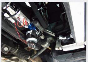
**Figure 2**: Mounting locations for temperature and pressure sensors. (Sensor reads approximately 10 times per second.)
