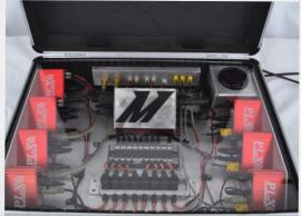
**Figure 3**: PLX sensor modules were used to monitor engine pyrometers.
