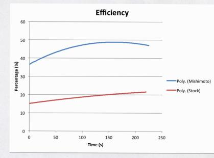
**Figure 8**: The Mishimoto oil cooler shows a 29% increase in efficiency.
