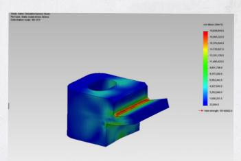
Figure 5: FEA stress testing of oil cooler mount
