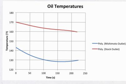
**Figure 7**: The Mishimoto oil cooler shows a 30° F lower outlet temperature compared to stock.
