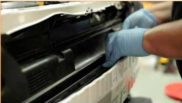
5. Install the optional self-tapping screws into the bottom of the oil cooler and secure it to the plastic under tray.
