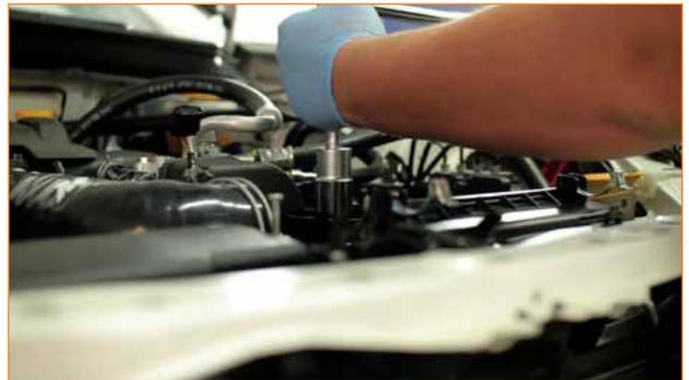
10. Install the oil lines onto the sandwich plate. Tighten down all the oil line fittings.
