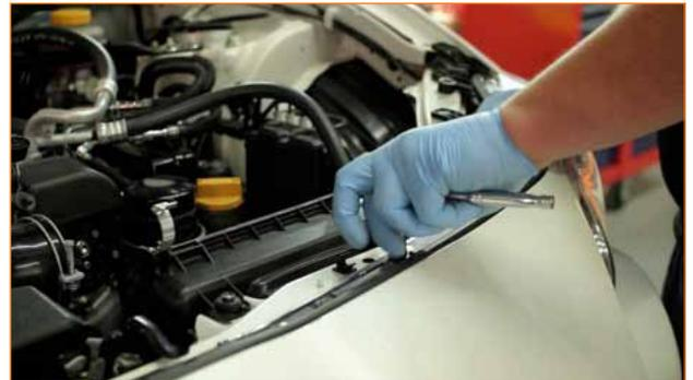
5. Remove the four pop clips from the inside of the fender on each side of the car. One pop clip is behind the corner marker light.
