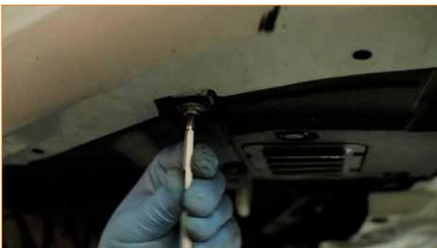
7. Reinstall the four pop clips on the inside of the fender on each side of the car.
