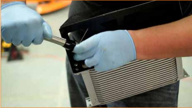
3. Install the Mishimoto oil cooler and feed the oil lines into the engine compartment.
