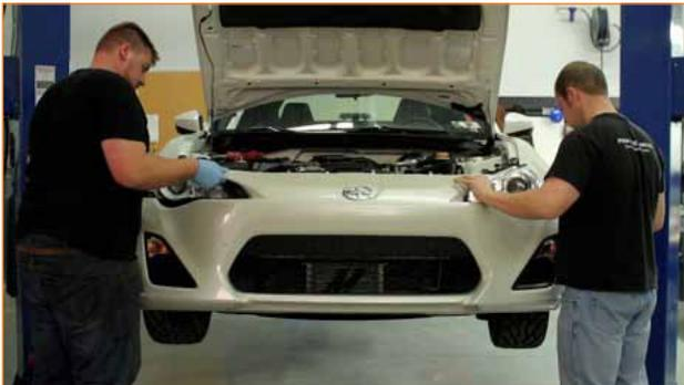
5. Reinstall the front splash shield with the three 10mm bolts and nine pop clips.
