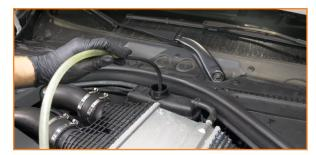
2. Disconnect the sensor on the side of the intercooler. Press the tab at the center of the connector to release the harness.
