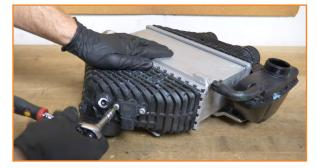
Compress the clamp on the small hose connecting the expansion tank to the intercooler. Slide the small hose off the intercooler port. (1x spring clamp)
