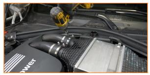
Separate the quick-disconnects from the intercooler. Lift the clip on each one to free the connections. Place something underneath to catch residual fluid from these connections. (3x spring clips)
