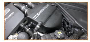
15. Reattach the quick-disconnects. (3x spring clips)
