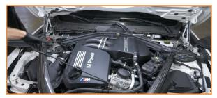
5. Lift the cover off the engine.
