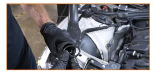
13. Attach a silicone coupler to the back intercooler pipe. Then set the back pipe on the turbo and slide the coupler onto the intercooler. (1x E11 torx bolt, 2x worm gear clamps)
