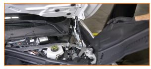
Remove the bolts that secure the front and ends of the strut bar. (8x 13mm bolts)
