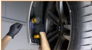
4. Pull back the wheel well liner to gain access behind it. Remove the bolts that secure the bumper to the edge of the fender. (4x 8mm bolts)
