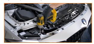
Remove all the bolts on the lower splash shields and wheel well liners.
