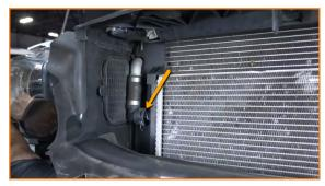
14. Remove the bolts that secure the oil cooler. (3x 13mm bolts)
