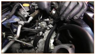
37. Route the hose toward the valve cover vent on the driver side.
