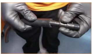
**34**. Attach the supplied Y-fitting and a worm-gear clamp to the opposite end of the hose from step 33. Tighten the clamp. (Flathead screwdriver)
