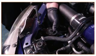
7. Remove the 10mm nut and then remove the front-side battery tie-down.
