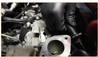
**38.** On the Y-fitting end, attach a worm-gear clamp to the valve cover vent hose on the driver side. Connect this hose to one side of the Y-fitting, Tighten the clamp. (Flathead screwdriver)
