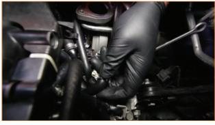
**31.** Attach a worm-gear clamp to the other end of the intake manifold hose from step 30, and then route the hose to the outlet on the catch can on the passenger side. Tighten the clamp. (Flathead screwdriver)
