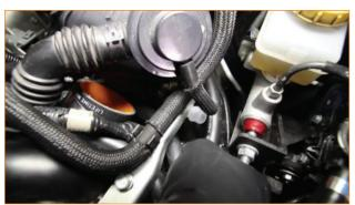
**39.** Attach a worm-gear clamp to the remaining hose coming from the second inlet on the catch can on the driver side. Connect this hose to the other side of the Y-fitting. Tighten the clamp. (Flathead screwdriver)
