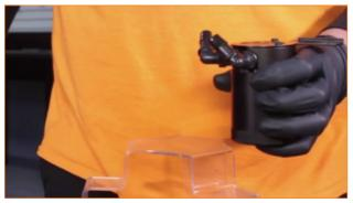
**5.** Thread and tighten the two fittings on the 2-port catch can. [11/16th" wrench]
