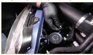
33. Attach a supplied plastic fitting and a worm-gear clamp to the longer of the two straight hoses. Tighten the clamp. (Flathead screwdriver)
