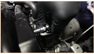
**15.** Remove the second 10mm bolt on the side of the head as shown below.
