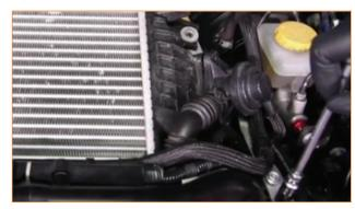
**12.** Remove the two 12mm bolts from the passenger side of the intercooler that connects to the turbo.
