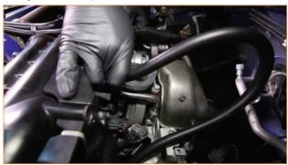
**30.** With a worm-gear clamp already installed on the hose, attach the next hose to the intake manifold. (Flathead screwdriver)
