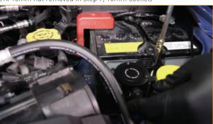
**9.** Loosen the worm-gear clamp on the throttle body hose. [10mm socket if you have a Mishimoto throttle body hose; flathead screwdriver if you have a stock throttle body hose]
