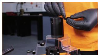
**3.** Attach the final direct-fit bracket to the 3-port catch can lid. (2x 2.5mm Allen bolts and washers, Allen key)
