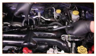
$\bf 24.$  Using a clamp, attach the L-shape hose to the outlet of the catch can on the driver side. (1x worm-gear clamp)
