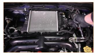
10. Remove the two 10mm bolts from the bypass valve (BPV).
