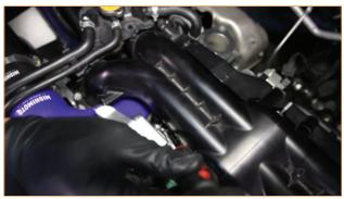
**21.** Shimmy the supplied L-shape hose into the space previously occupied by the hose that was removed in step 20. Tighten the worm-gear clamp. (Flathead screwdriver)
