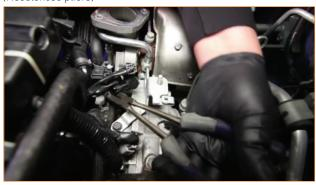
29. In the same spot, attach a worm-gear clamp to the next hose and tighten the clamp. (Flathead screwdriver)
