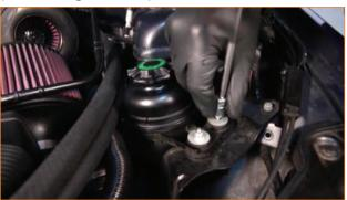
22. Using the two 10mm nuts removed in the previous step, install the catch can assembly onto the bracket and tighten the nuts.
