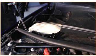
10. Remove the six 8mm course-threaded bolts that hold the cabin filter to the main panel, and then remove the cabin filter.
