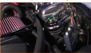
23. Connect the hose coming from the valve cover to the inlet on the catch can. (These hoses are under vacuum, so worm-gear clamps are not required.)
