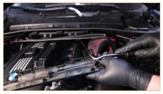
4. Remove the last wire harness. Unfasten the two clips and pull outward.
