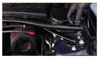
6. Twist the harness on the passenger side about 30 degrees and pull outward. Set the harness aside.
