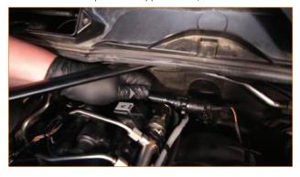
14. Unclip the other side of the flapper valve, and then remove the entire hose. (Pick tool or screwdriver)
