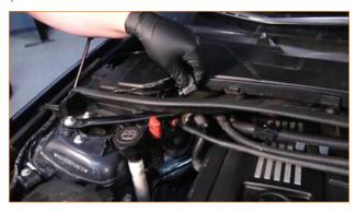
7. Remove the passenger-side panel by lifting up on the two side tabs and moving the last tab toward the cabin of the vehicle.
