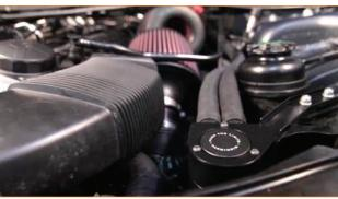
25. Reinstall the engine cover. (4x Allen bolts)
