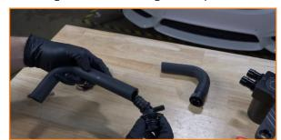
16. Install the larger hose and reconnect the electrical connector to the heater block. Secure it with the plastic screw. (1x T25 torx)
