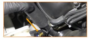
12. Remove the two fittings from the stock hose. Apply heat to loosen the fittings and slide them out of the hose.
