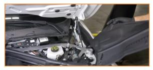
2. Remove the bolts that secure the front and ends of the strut bar. (8x 13mm bolts)
