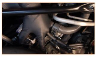
**4.** Remove the 1x 12mm nut from the driver-side shock-tower brace.
