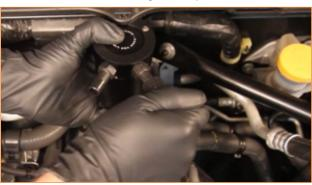
**13.** Install the silicone hose that runs from the out port on the catch can to the intake manifold. (2x worm-gear clamps)
