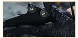
Install the Mishimoto catch can bracket using the original hardware from the stock bracket. Make sure to attach the power steering fluid container to the available slot on the Mishimoto bracket. (2x 10mm bolts)
