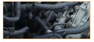
Install the larger hose to the intake manifold and OUT port on the catch can. Run this hose under the electrical harness near the engine port. (1x 12-20mm worm gear clamp, 1x 16-25mm clamp)
