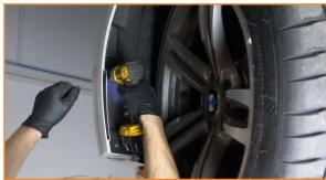
Pull back the wheel well liner to gain access behind it. Remove the bolts that secure the bumper to the edge of the fender. (4x 8mm bolts)
