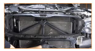
13. Separate the quick-disconnects along the passenger side of the heat exchanger.
