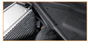
Loosen all the clamps on the intercooler pipes. (5x worm gear clamps)
