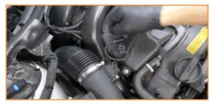
8. Remove the bolt that secures the remainder of the intake to the turbo. With the intake now free, remove it from the engine bay. (1x 10mm bolt)
