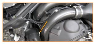
7. Disconnect the MAF sensor. Depress the black tab at the center to release the connection. Then lift the airbox out of the way.
