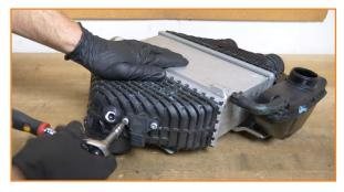
Compress the clamp on the small hose connecting the expansion tank to the intercooler.
