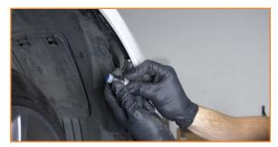
6. Disconnect the electrical harness within the wheel well.
