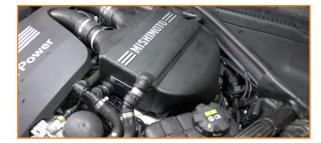
15. Reattach the quick-disconnects. (3x spring clips)
