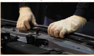
**6.** Remove the three small fender clips located in both the passenger and driver side fender wells.
