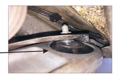
OE ball joint shown - re-use OE flange nuts only - tighten to OE specification.
