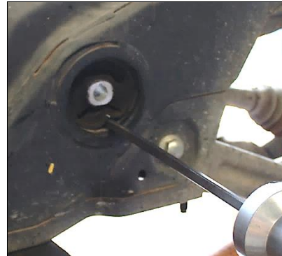
Figure 2 – Removal of differential outrigger bush
