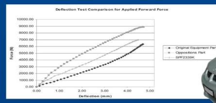
Note the high forces displayed on the other part, and the digressive nature of the graph, this means the POSSIBILITY OF TRANSMITTING NVH (Noise, Vibration and Harshness).
